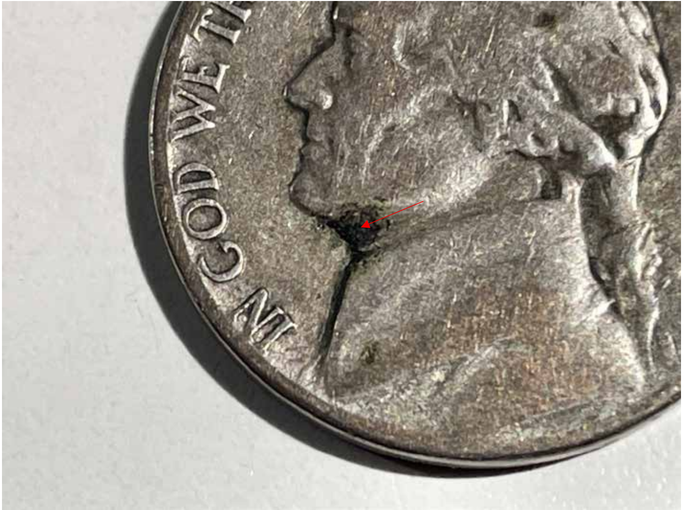
Figure 1: Jefferson Nickel. 1943-S 21.13 mm, 4.73 grams. The manganese-oxide concentration beneath Jefferson's chin (red arrow pointed area) on this 1943-S war nickel represents a classic early-stage surface failure zone in the wartime Cu–Ag–Mn alloy. In this region, Mn-rich oxides have migrated toward the surface and begun forming brittle, darkened patches that sit within the surrounding metal. These oxide clusters often mark the initiation point for micro-lifting and shallow delamination because the Mn-oxide phase bonds poorly to the copper-silver (Cu/Ag) matrix. The spot you're seeing is essentially the visible expression of that weak interfacial chemistry—an area where the alloy's internal instability is beginning to break through the surface. Under a stereo microscope at 40-50X the Mn-oxide appear as individual circular spheres all tightly agglomerated together as seen by this author in this location under Jefferson's chin area.
