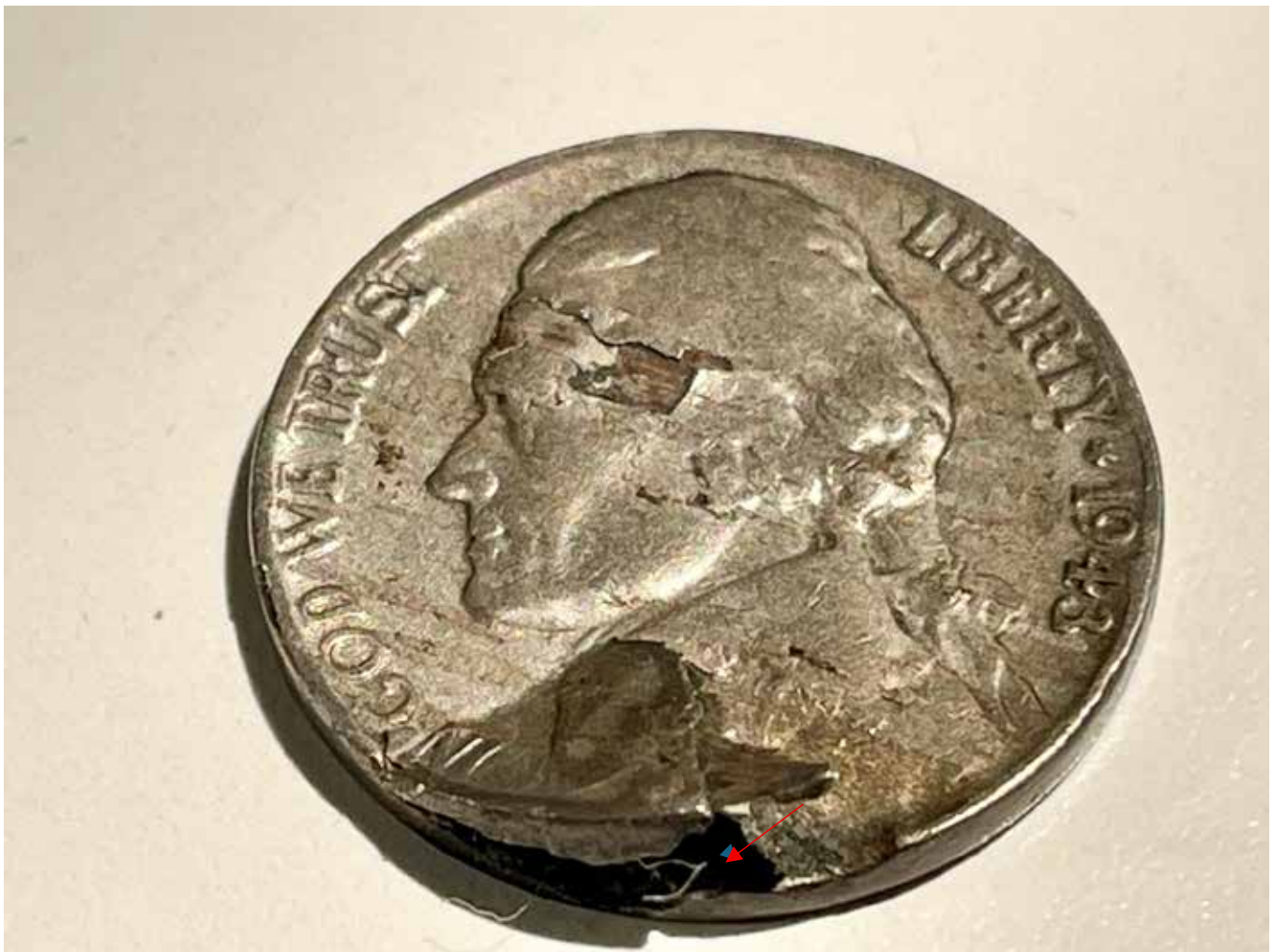
Figure 3: A massive almost peeled away area in the lower part of the obverse.
