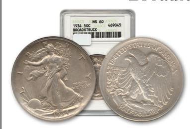
broadstruck error occurs when a coin is Astruck without the collar to form the rim and edge that is part of the shape of the coin. Coins can be broadstruck on either type one or type two planchets. When a coin is broadstruck the blank being fed into the collar will spread and distort outward as it is being struck because the collar isn't in the correct position to retain it.
