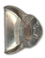
Afold-over coin is one of the most dramatic types of errors. It occurs when the blank is standing vertically between the dies. During the strike, the force is so great that it bends and folds the blank. These fold-overs can be on-center or off-center, and come in many different shapes. There are a few fold-overs with multiple errors, either with an additional strike or fold-over. Denominations above quarters are very scarce.
