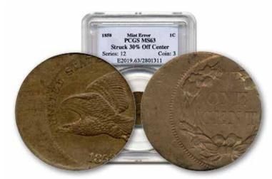
Off-center coins are one of the most common and best known types of errors. This happens when a blank which is supposed to be fed into the press, lands in the collar improperly. When this occurs only part of the blank is between the upper and lower dies. When the dies strike the blank, only that part will be struck with a design.
