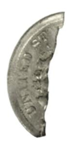
The blanking press takes the coils of metal strips and punches blanks out of it, ejecting the webbing at the other end. The webbing is cut into small scrap pieces to be melted and recycled. Occasionally a scrap piece will be mixed with the blank planchets and struck by the dies. Struck fragments are rare in the larger denominations. These can be uniface or die struck both sides and are very rare on type coins.
