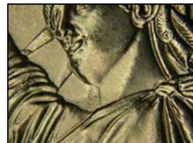
4a.) Minor die damage visible near Liberty's neck, as shown, is not significant enough to be considered a mint error and is not noted on the holder by NGC.
