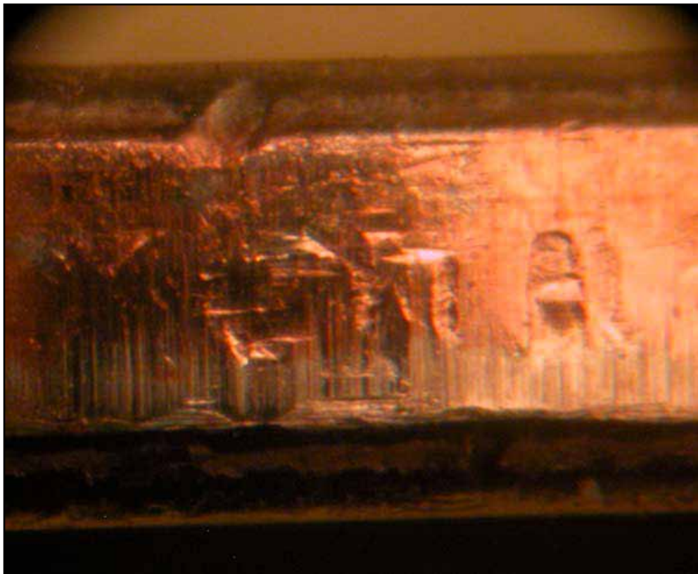
Photo 2: This is a genuine Washington dollar with the edge lettering missing. The surfaces are original and unaltered and also show the fine vertical ejection marks.
